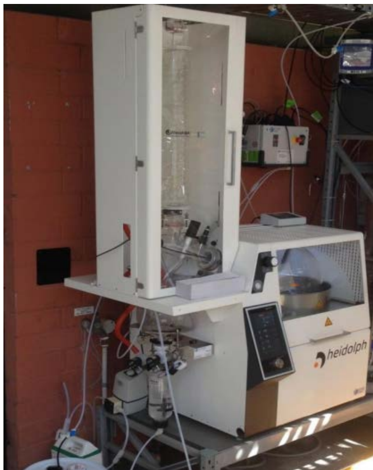
Figure 3-2. Curtin Corrosion Centre MEG reclamation system
