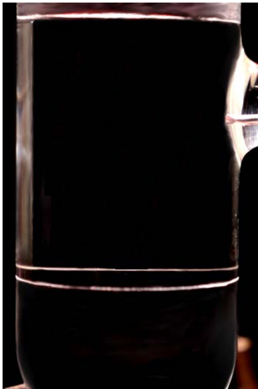
Figure C-4. Settlement of water/MEG-wetted \text{FeCO}_3 ( >63 \mu\text{m} ) in 50% wt. MEG solution
