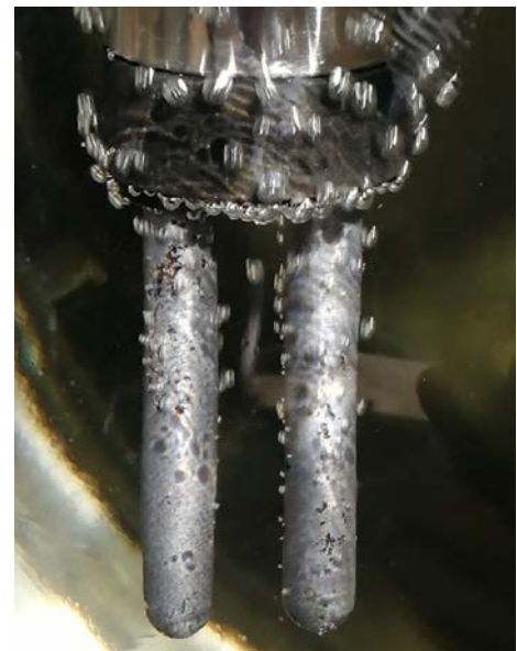
Figure 6-7. Corrosion of LPR probe during regeneration (pH 25°C = 7, 140°C)
