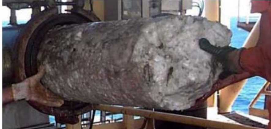
Figure 2-2. Gas hydrate plug in pipeline (Makogon [26])
