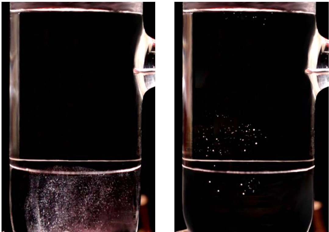
Figure C-5. Comparison of water/MEG-wetted and oil-wetted quartz (>63 \mu\text{m} ) in 50% wt. MEG solution
