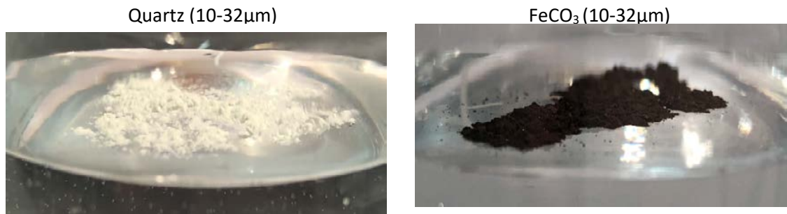
Figure C-1. Behaviour of oil-wetted solid particles at MEG-air interface
