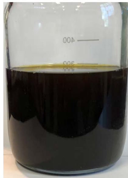
Figure 6-10. Final solution after 3-days of corrosion (pH 25°C = 7, 140°C)
