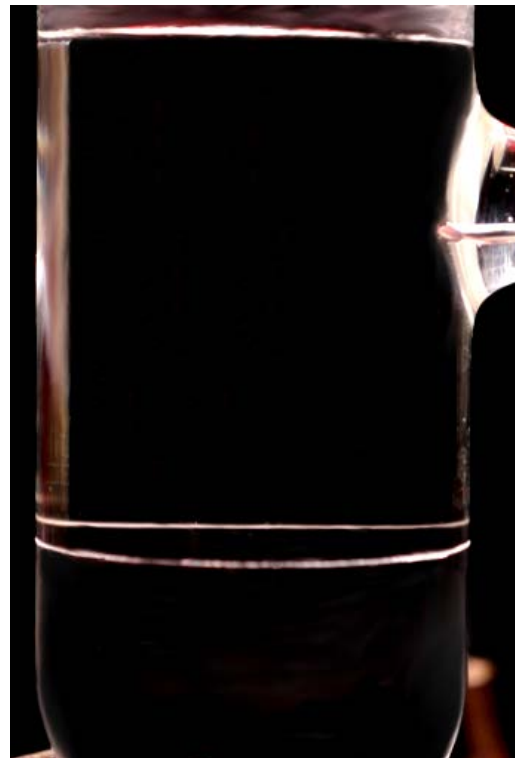
Figure C-4. Settlement of water/MEG-wetted \text{FeCO}_3 ( >63 \mu\text{m} ) in 50% wt. MEG solution
