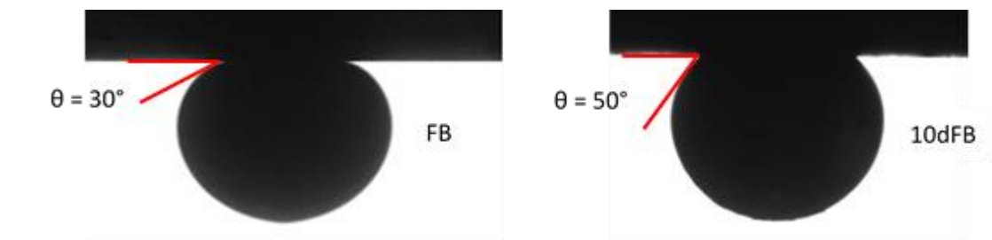
Figure 3-3. Contact angle of various brine and oil on the carbonate (un-aged) sample.
