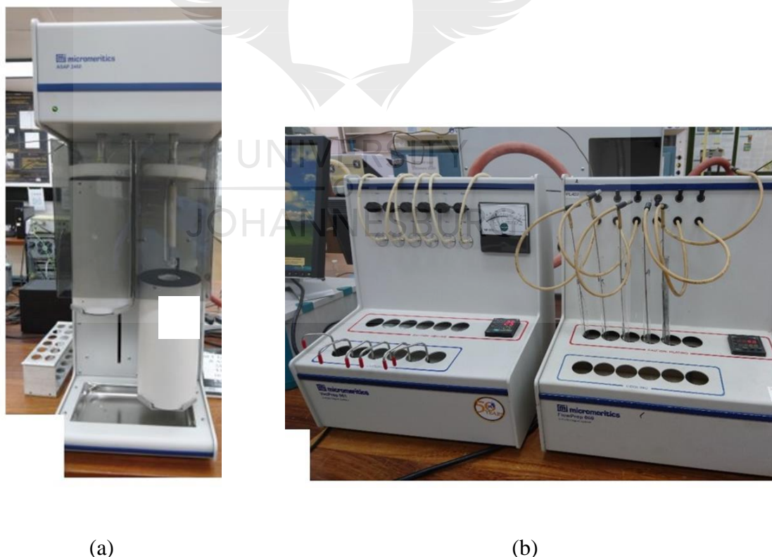
Figure 3.21 Nitrogen sorption porosimetry. (a) BET equipment; (b) Degassing equipment
