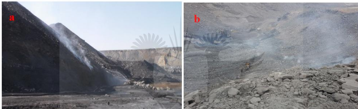
Figure 2.1 (a) Self-heating of stockpile and (b) symptoms of self-heating within coal seam, Witbank Coalfields, South Africa (Onifade, 2018)
