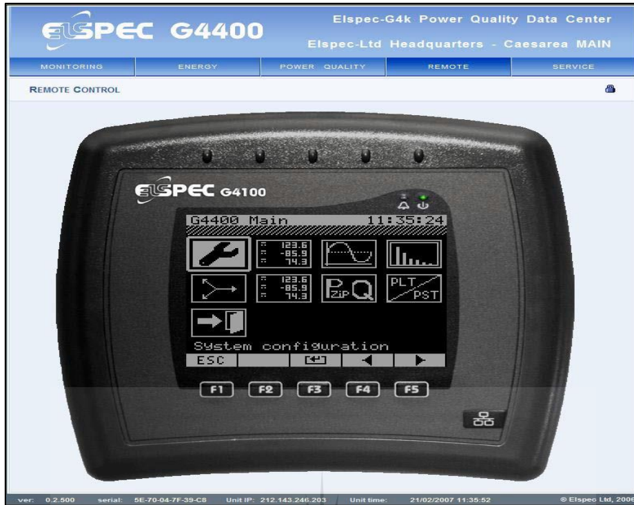
Fig. 5.3: Web based remote display unit
