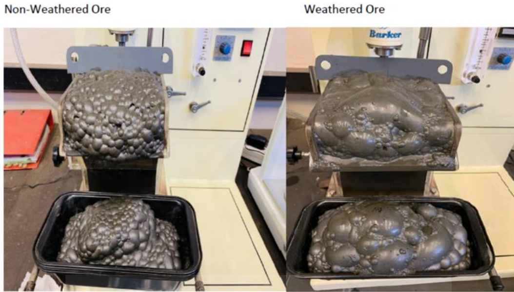
Figure 4.11: Bubble sizes and colour during flotation pristine and weathered ore
