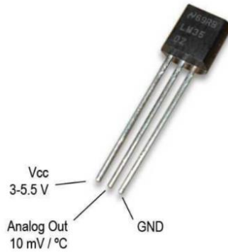
Figure 3.8: LM35 temperature sensor [56]
