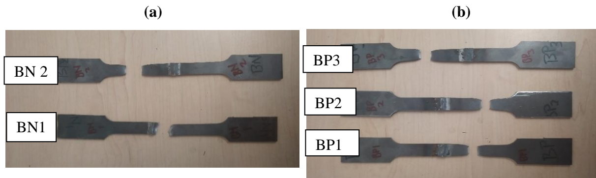
Figure 4-27: Fracture of butt welds a) unreinforced samples b) reinforced samples
