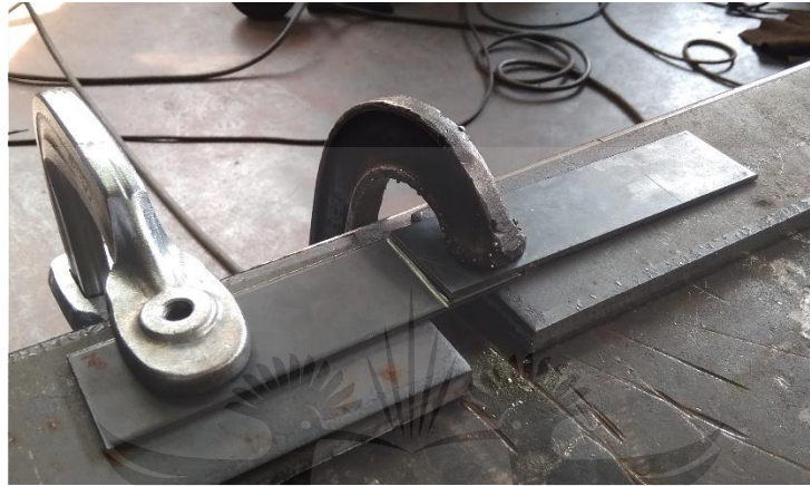
Figure 3-4: Set up for lap joint configuration
