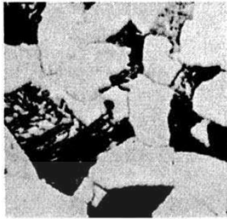
Figure 2-17: Ferrite and pearlite in 0.4 wt. % C steel [77]
