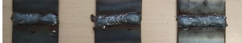
Figure 4-1: Visual Inspection of Butt Joint Welds
