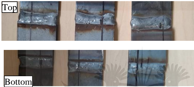
B) Sample L2, welded at 23V, 240A with titanium 6-2-2-2 alloy reinforcement
