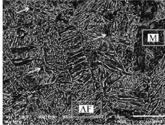
Figure 2-37: SEM Micrograph for GMAW HSLA naval grade steel sample, Weld Metal [30]
