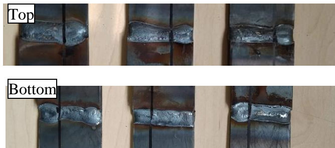
D) Sample L4, welded at 26V, 240 A with commercially pure Ti reinforcement
