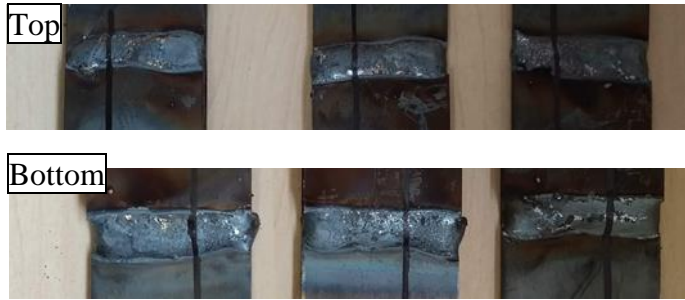
A) Sample L1, welded at 23V, 215A with commercially pure Ti reinforcement.
