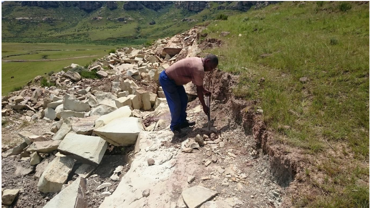
Figure 4.7: Visual image of the top soil removed before the extraction of sandstone.
