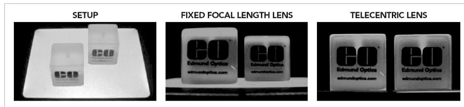
Figure A.10: The angular field of view of the Fixed Focal Length Lens translates to parallax error in the image and causes the two cubes to appear to be different sizes.
