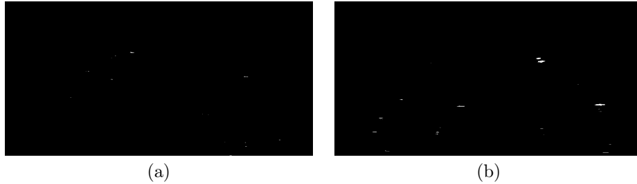
Figure 8.5. Simulated diffraction patterns of Test Case II in the absence of noise. Intensities have been binarized for easier visibility; black pixels denote a photon count of zero, white ones have a positive photon count. Only the lower third of the total detector area is shown; the rest is completely black. The non-diffracted incident X-ray beam passes just below the lower side of the detector (not indicated). (a) Projection at \omega = -43^\circ . (b) Projection at \omega = 27^\circ .
