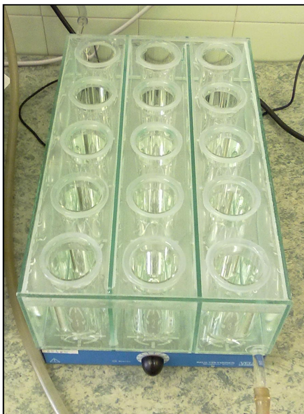
Figure 9: The custom-made solubility apparatus
