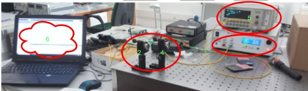
Figure 5.1: Experimental setup for indoor optimization of an automatic FSO alignment system.
