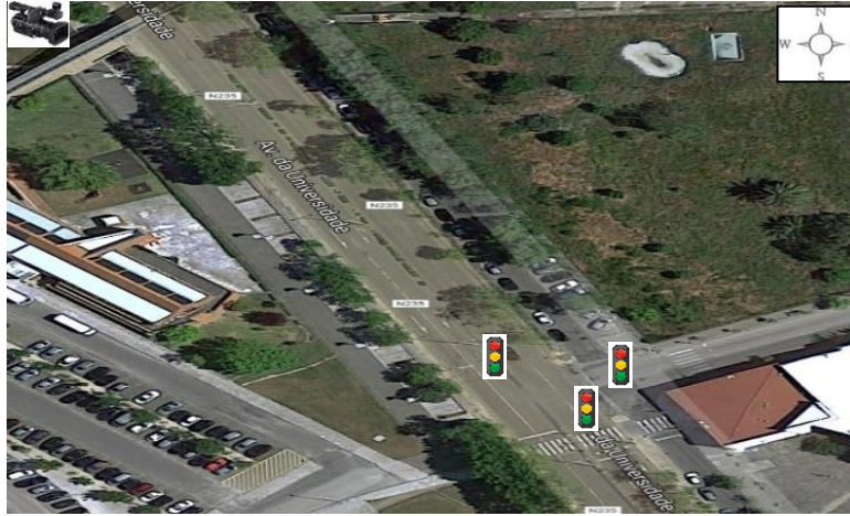
Figure 3.2. Layout of the case study with the identification of videotaping and traffic lights. (Source: http://www.bing.com/maps/ )
