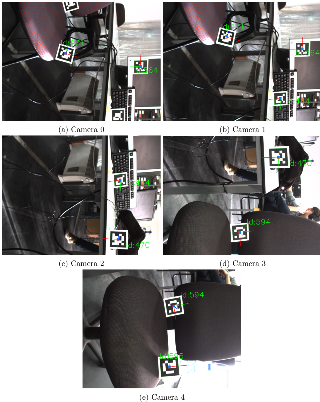
Figure 5.16: Representation of dataset 3 and the markers' center (red squares) and reprojection of the 3D points on the image using the initial guess (blue squares).
