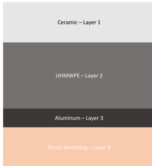
Figure 4.3: Sketch of the different layers for the new helmet concept.
