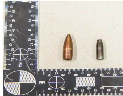
(b) 7.62 × 39 mm projectile (left) and steel core (right).
