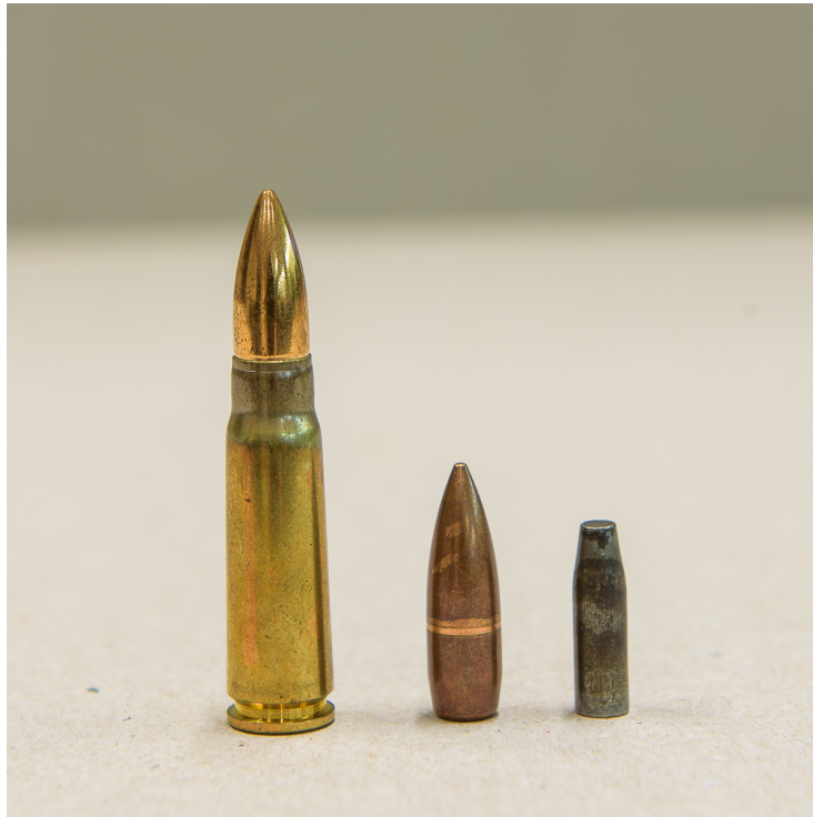
Figure 4.2: 7.62 \times 39mm (from left to the right): ammunition cartridge, projectile and steel core.
