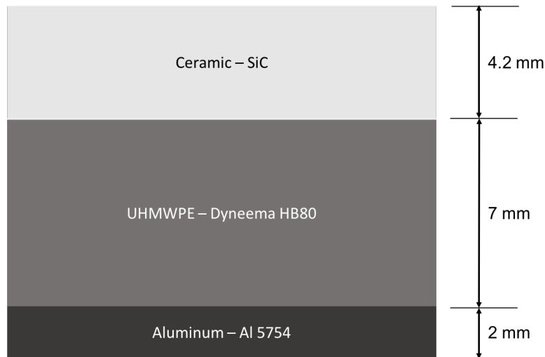
Figure 7.29: Schematic model for the first three layers of the new helmet concept (SiC, Dyneema HB80 and the Al 5754 - H22).
