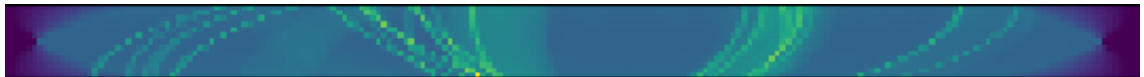
Figure 22: An example sinogram of a simulated phantom, with each row being one measurement from 13 evenly distributed angles within a field of view of 40 degrees.
