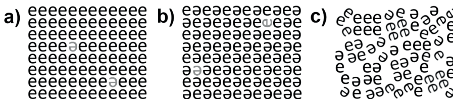
Figure 1. A schematic representation of different forms of a substance with the same chemical composition. A) crystalline stable form I, b) crystalline metastable form II and c) unstable amorphous form. The letter e represents a single molecule. Crystal defects in crystalline materials have been illustrated using grey color.
