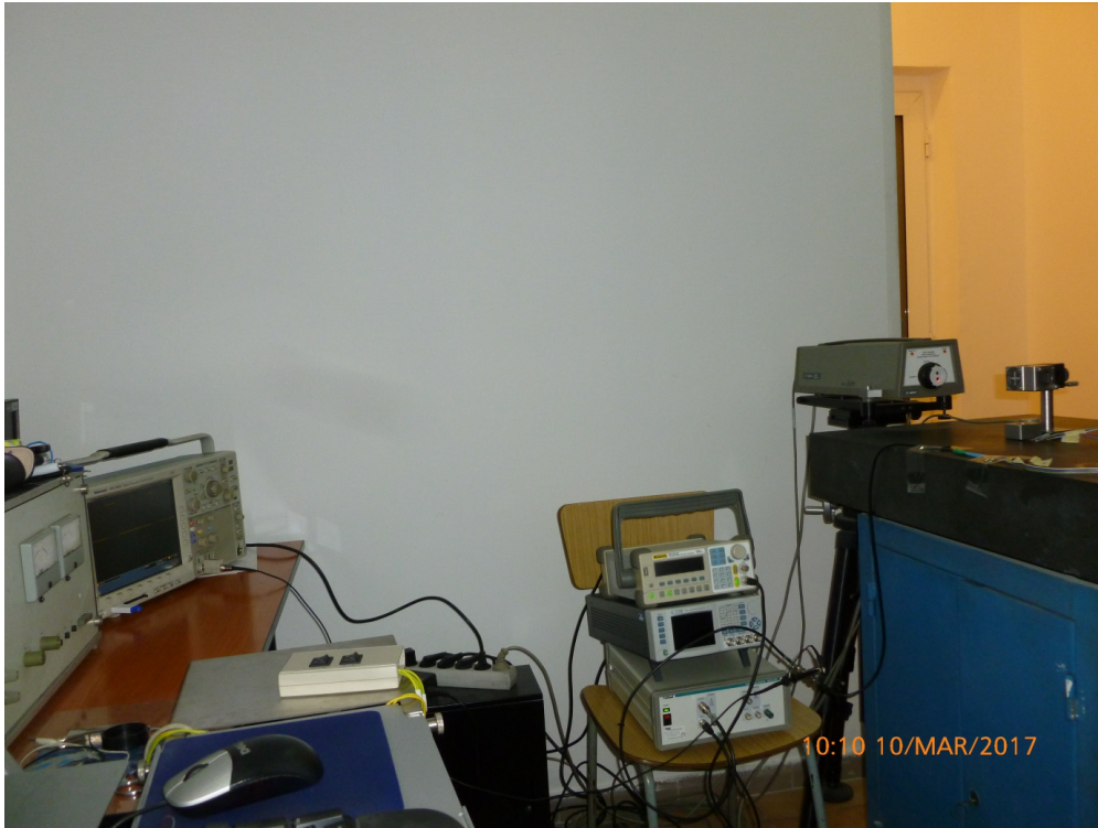
Figure 4.3: Laboratory setting used in the interferometric testing performed in the Micro-nano Technologies Laboratory of the institute INCDIE ICPE-CA . From left to right, the oscilloscope, the arbitrary waveform generators, the amplifier, the interferometer, the piezoelectric patch and the support table with the granite block can be seen.
