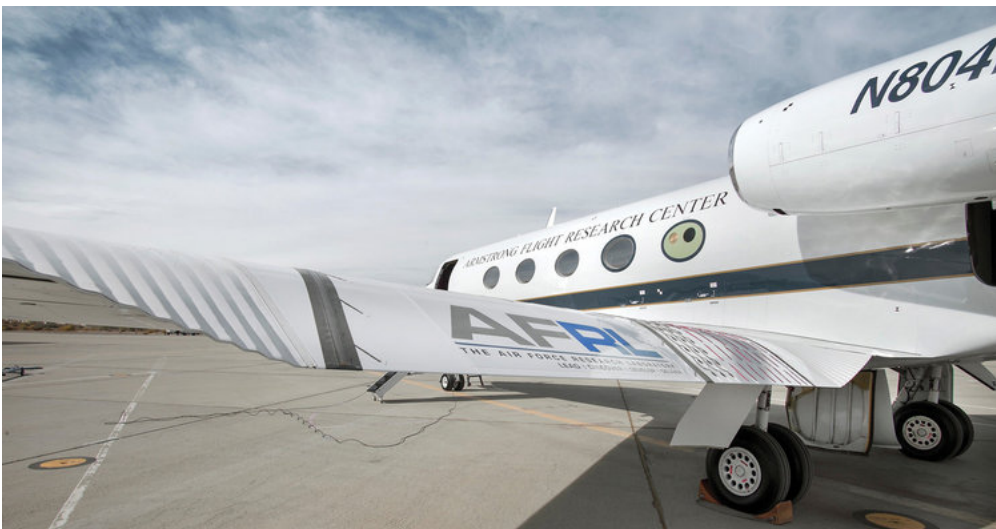
Figure 1.6: Flexfoil system integrated in a NASA Gulfstream 3 for flight testing during 2018.
