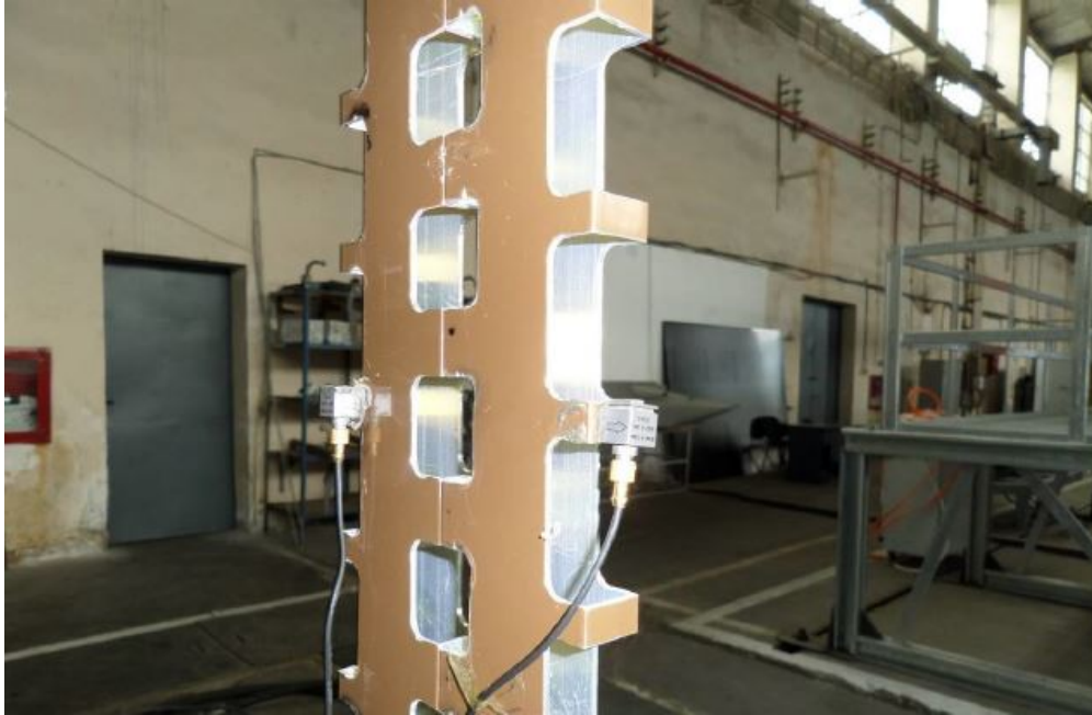
Figure 6.17: Detail of the positioning of the accelerometers for one of the tested configurations.
