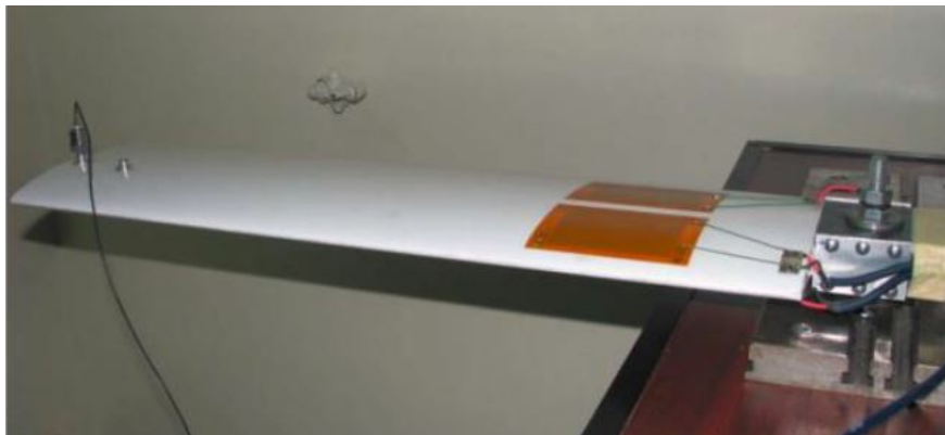
Figure 6.11: Equivalent system used in the development of the receptance-based control algorithm.
