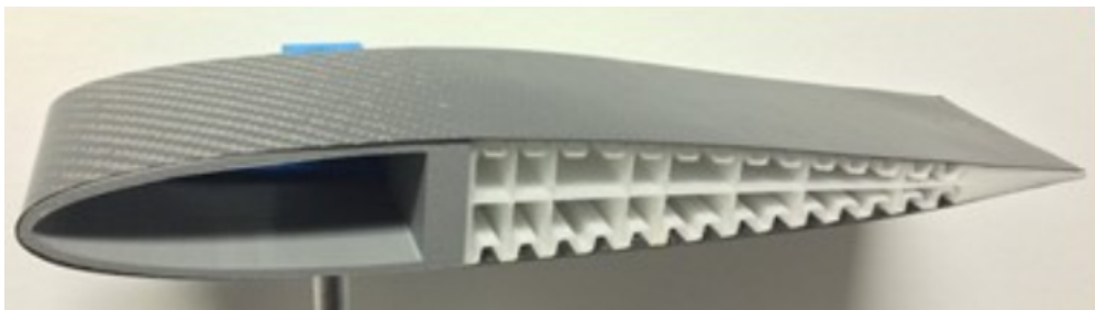
Figure 1.10: Example of a piezoelectric driven wing profile morphing application with rigid leading edge and flexible trailing edge. [76]
