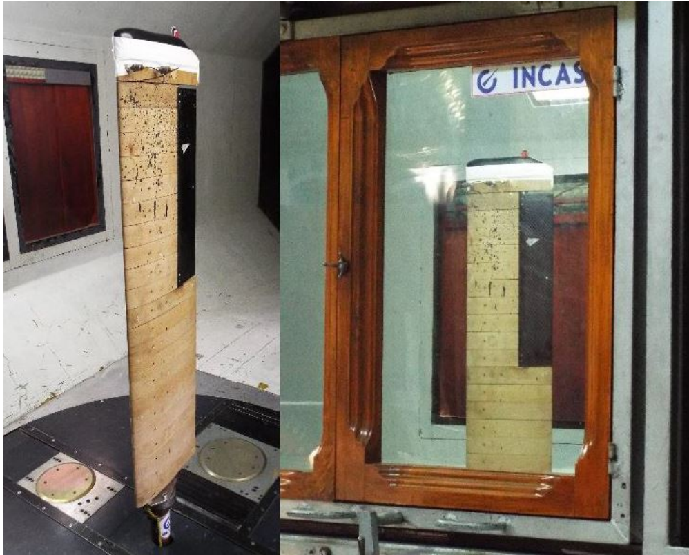
Figure 6.31: Positioning of the AFDPA system in INCAS's subsonic wind tunnel.
