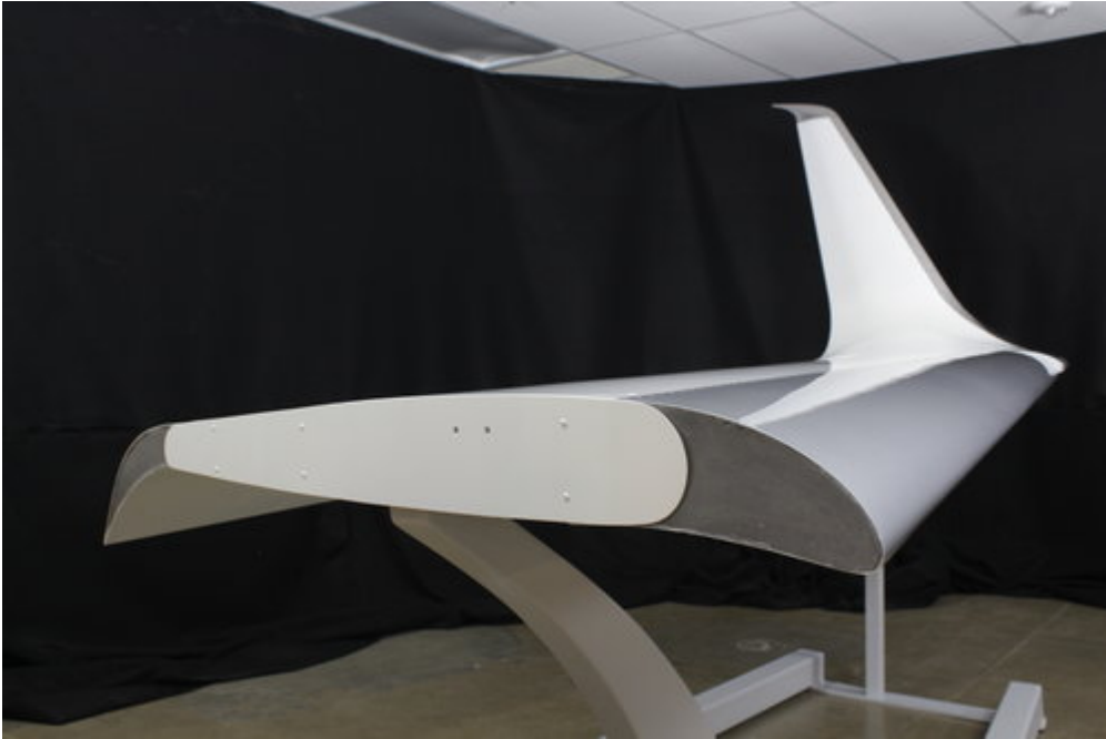
Figure 1.5: Flexfoil ground demonstrator showing the deformation capability for both leading and trailing edge devices.
