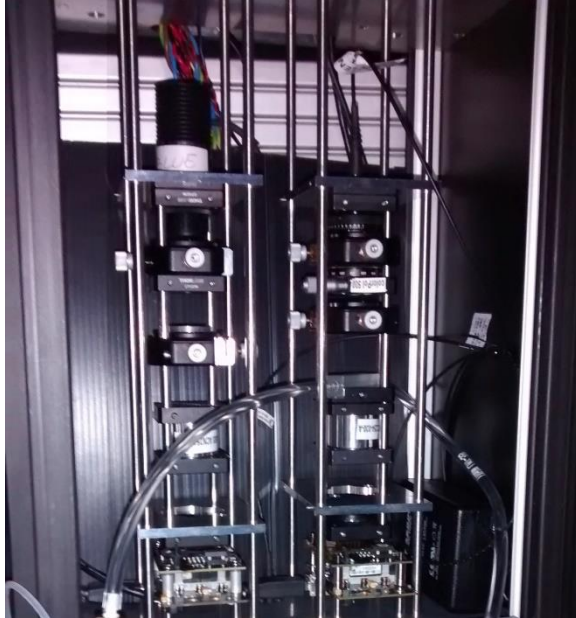
Figure 2.1: Photo of two early laboratory implementations. This was an alpha prototype in which two different optomechanical assemblies were built. Both implementations used an achromatic optical lens of 30mm focal length as an optical transforming element and microlens arrays of 10mmx10mm with a 300 \mu m pitch and 18mm focal length. The difference between implementations was in the light source used. On the left side of the image we see a prototype built with a free space LED. On the right side of the image we see a prototype built with a fiber optic coupled LED.
