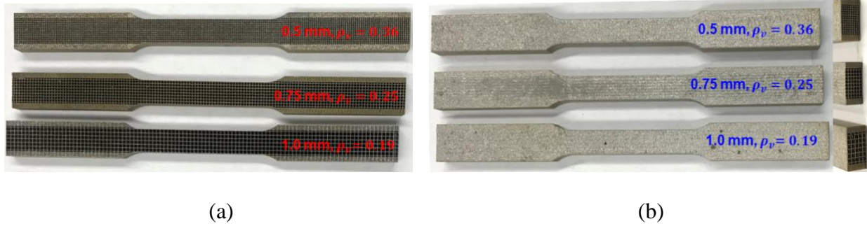
Figure 4.6 Tensile Specimens of Thin-Walled Lattice Structures Fabricated (a) Horizontally and (b) Vertically by DMLS
