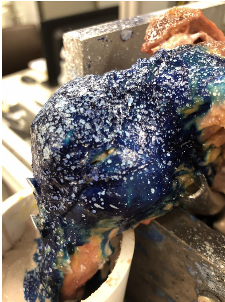
Figure 10. A specimen stained with dye and speckled with paint
