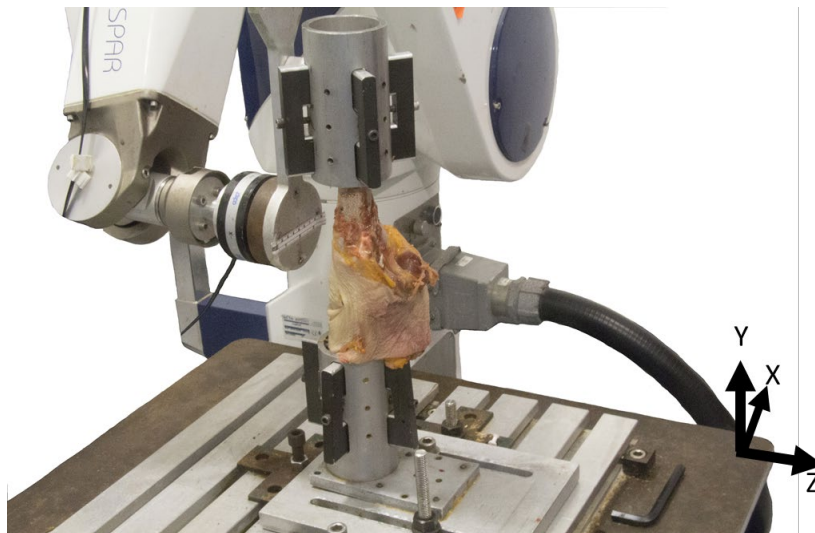
Figure 6 – Set up of robotic system, with the femur rigidly fixed and the tibia attached to the robot end-effector.
