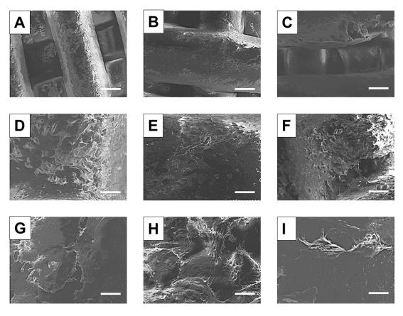
**Figure 9.** SEM micrographs of U2OS cells seeded on PCL (**A,D,G**), PCL/10Sr-nHA (**B,E,H**) and PCL/20Sr-nHA (**C,F,I**) after 14 days in culture; ((**A–C**) scale bar = 200  $\mu$ m; (**D–F**) scale bar = 40  $\mu$ m; (**G–I**) scale bar = 8  $\mu$ m).
