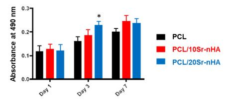
**Figure 7.** Absorbance values of the MTT assay evaluated up to 7 days for PCL, PCL/10Sr-nHA and PCL/20Sr-nHA scaffolds in culture with U2OS cells (data are presented as mean  $\pm$  standard deviation; n = 3, p < 0.05 (\*)).
