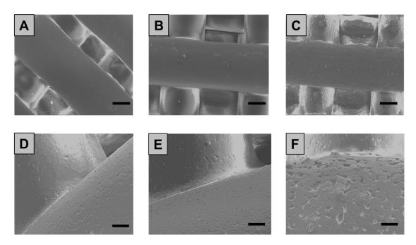
**Figure 4.** SEM images of the 3D printed PCL (**A**,**D**), PCL/10Sr-nHA (**B**,**E**) and PCL/Sr20-nHA (**C**,**F**) scaffolds ((**A**-**C**) scale bar = 200 µm and (**D**-**F**) scale bar = 50 µm).
