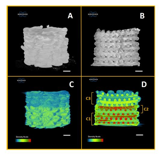
**Figure 5.** microCT reconstructions of: **(A)** PCL scaffold, **(B)** PCL scaffold cross section, **(C)** multi-layer PCL/Sr-nHA scaffold and **(D)** multi-layer PCL/Sr-nHA scaffold cross section where the C1, C2 and C3 compartments are indicated.
