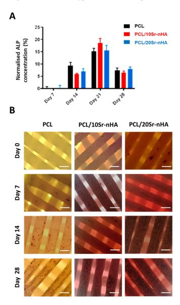
**Figure 10.** (**A**) Normalized ALP activity of the PCL, PCL/10Sr-nHA and PCL/20Sr-nHA samples up to 28 days in culture with U2OS cells (data are presented as mean  $\pm$  standard deviation. n=6) and (**B**) optical microscopy images of cell-seeded scaffolds showing calcified nodules stained with Alizarin red after 0, 7, 14 and 28 days (scale bar =  $400 \mu m$ ).
