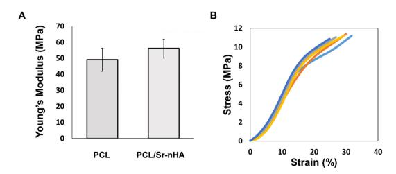
**Figure 6.** (**A**) Young's modulus values for PCL and PCL/Sr-nHA multi-layer scaffolds and (**B**) representative stress/strain curves (n = 5) for PCL/Sr-nHA multi-layered scaffolds tested in compression.
