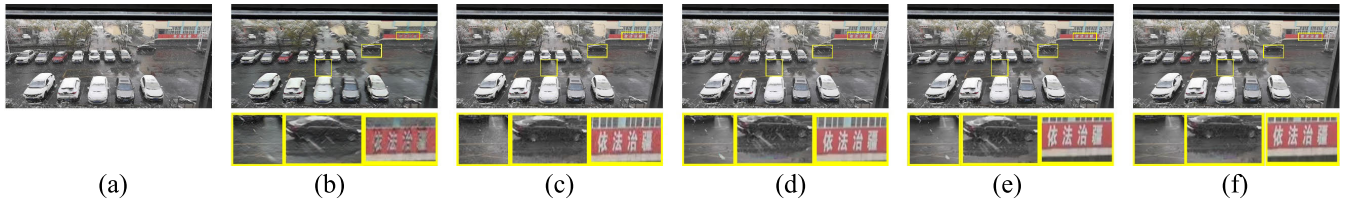
FIGURE 11. Comparison of the snow removal effects for frame 16 of the real video called “car”: (a) input; (b) Yang’s method [37]; (c) Kim’s method [9]; (d) Wei’s method [3]; (e) Li’s method [2]; (f) the VSRSG algorithm.
