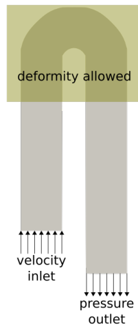
Figure 5. Position of inlet and outlet boundaries and the area where the geometry was a subject to change.
