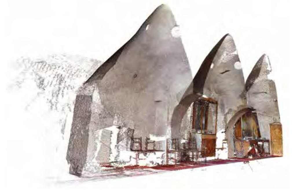
Section of a series of domes of the St. Tawadros Monastery (3D pointcloud, SfM). Compiled by B. Miklós based on data captured in 2017-2018.
