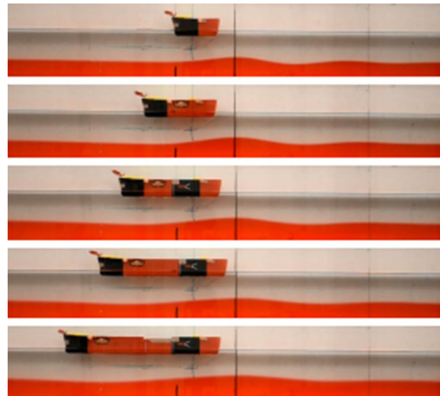
Fig. 4 The five different ship configurations of increasing length d , marked S_1 – S_5 (downward. cf. Table 2). The bottom layer is visualized using red food dye. The snapshots are organized such that the first wave trough locations behind the ship models are underneath each other
