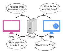
Figure 2.2: The working of a proxy server.
