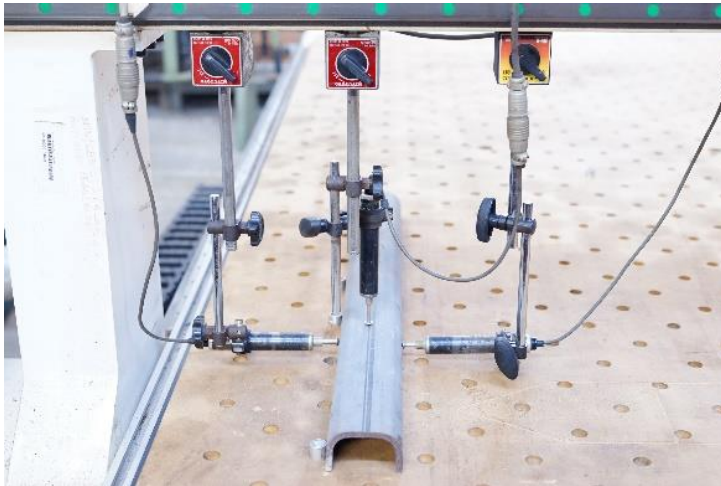
(b) Setup for initial local geometric imperfection measurements
