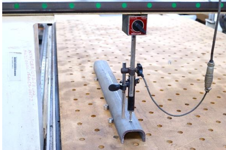
(a) Setup for initial global geometric imperfection measurements
