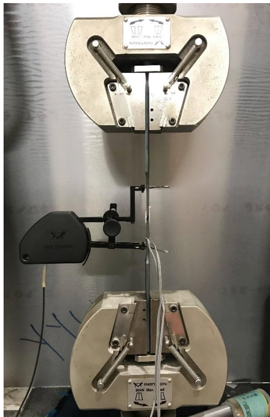
Fig. 4. Material tensile coupon test setup.
