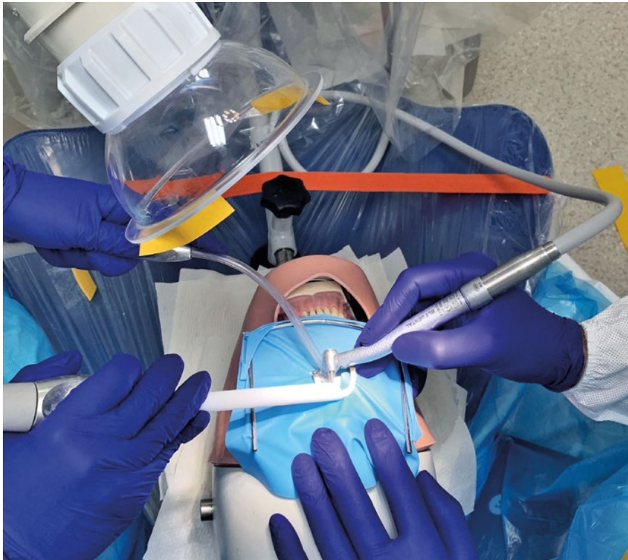
Fig. 3 Photograph showing procedure setup with location of EOS in 5 o'clock position above the dental manikin at 0.15 m distance
