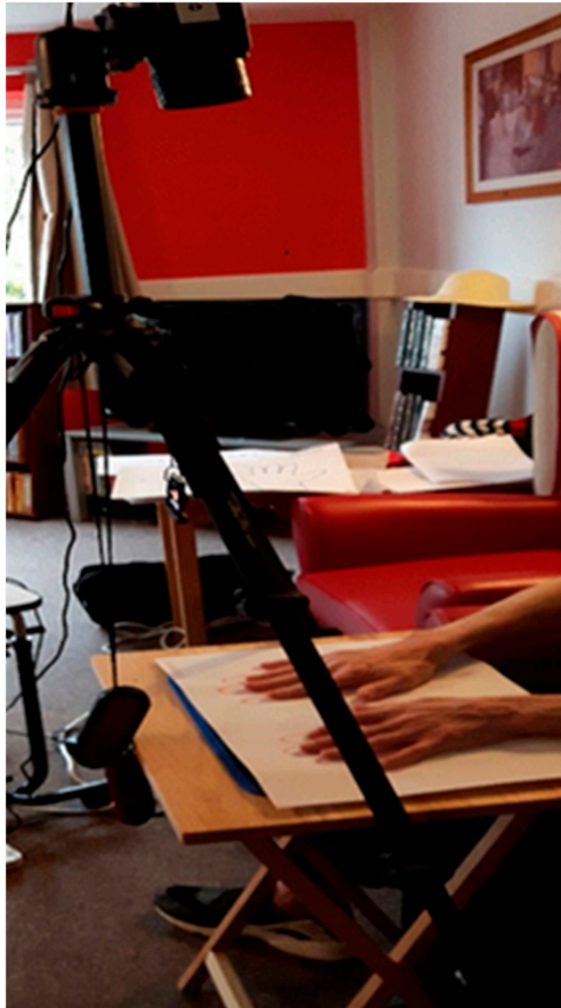
Figure 1. Long wave infrared imaging detector mounted on a tripod. The figure shows the participant during imaging with hands positioned upon a paper ‘hand template’ overlying an insulated tile. The portable table was used throughout the study to ensure consistency of the imaging set-up.
