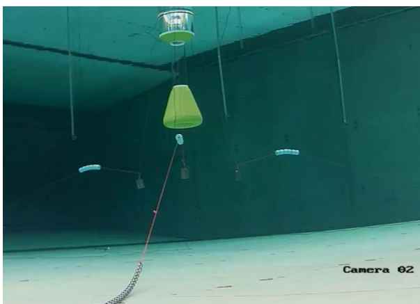
Figure 5: Underwater view of the mooring arrangement of the isolated device setup.
