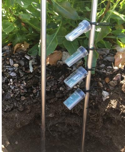
Figure 1.1 HOBOware temperature sensor set up: four sensors secured to a steel rod in air 5 cm above the wrack, on the wrack surface (0 cm) and at 5 cm and 10 cm depth into the wrack. (Photograph by E. Tully).
