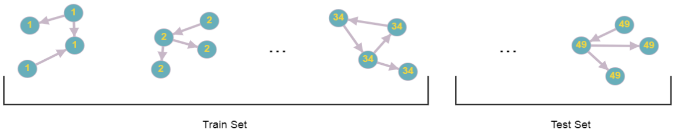
Figure 1: Abstract representation of train/test sets split of Elliptic data set. Nodes labelling represent the time-steps. Each connected graph has a unique time-step.
