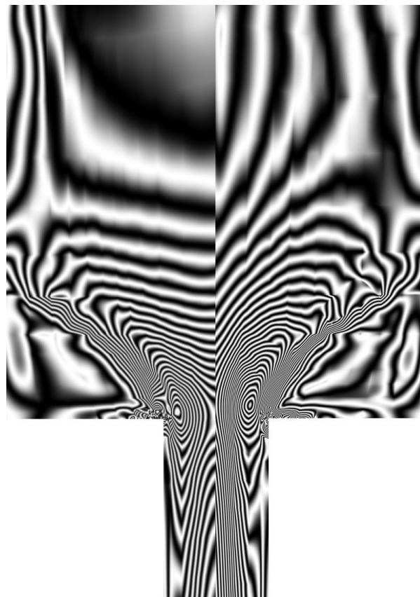
Figure 16 Comparison between 5:3 aspect ratio 3-D predictions (left) and 2-D predictions (right) at 73.7 g/min using convective constraint release mechanism CR2
