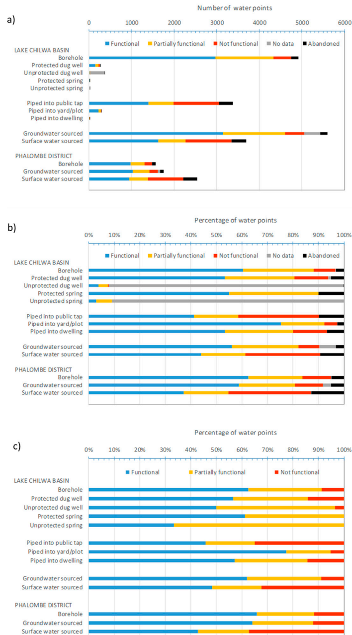
Figure 13. Water point functionality breakdown of Lake Chilwa Basin and Phalombe District subset surveyed in 2019 (based on mWater data retrieval May, 2020) showing: (a) numbers of water points; (b) percentage functionality across all five functionality categories; (c) percentage functionality across functional partially functional and not functional categories (three categories).
