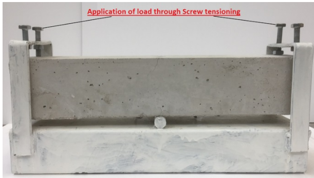
Fig. 1. Flexural method was used to create the crack in concrete sample
