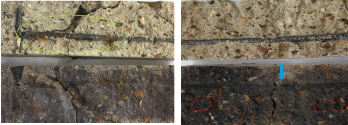
a: M 0.6 -cracked 0.25 mm (Carbonated )
