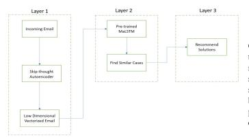
Fig. 5. DeepTMS - Ticket Management System Block Diagram
