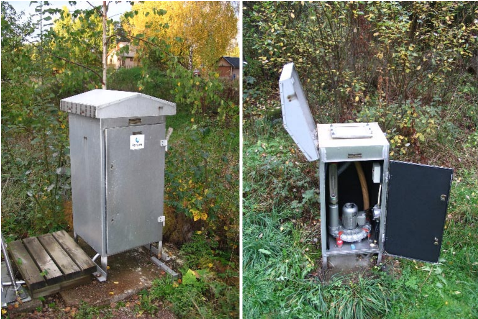
Figure 9. Stationary high-volume air samplers located in Loviisa and Olkiluoto.
