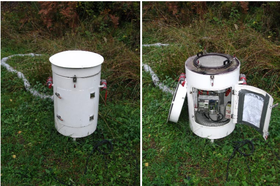
Figure 10. The supplementary portable high-volume air sampler.
