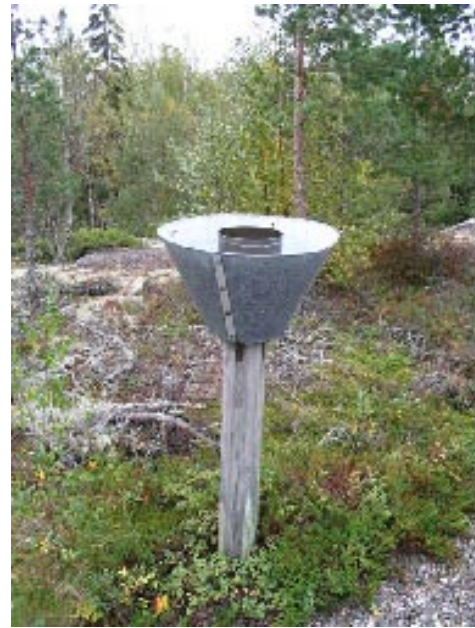
Figure 15. The collector for tritium in rainwater at Olkiluoto 21.
