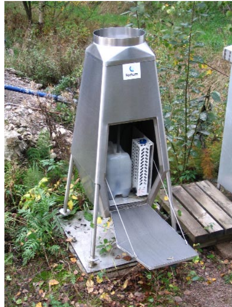
Figure 13. The “Ritva” collector for deposition. This collector is warmed in winter.
