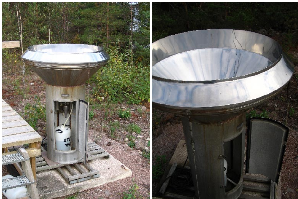
Figure 11. The large area collector for deposition at Loviisa.
