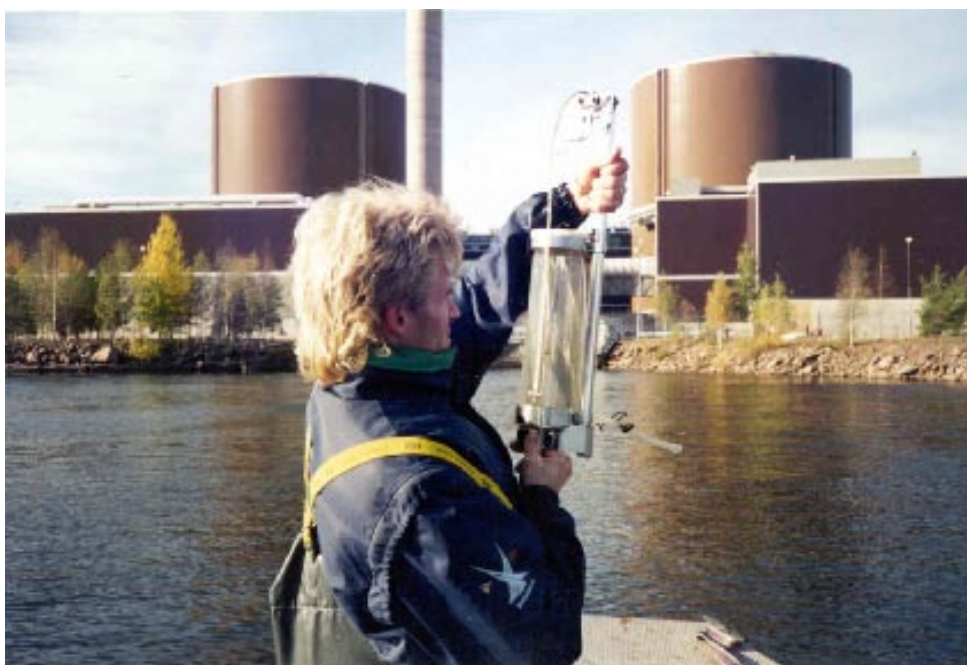
Figure 21. Water sampling with Limnos sampler.
