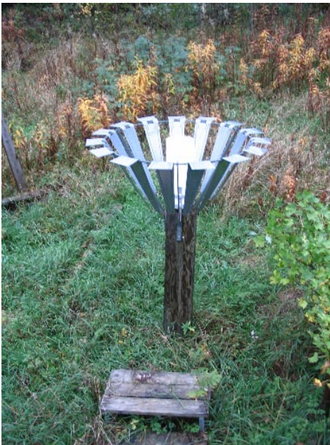
Figure 14. The collector for tritium in rainwater at Loviisa 33.
