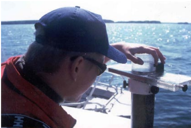
Figure 26. Slicing of a sediment sample with the sectioning apparatus of Gemini Twin corer.
