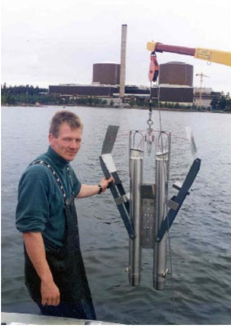
Figure 24. The Gemini Twin Corer.
