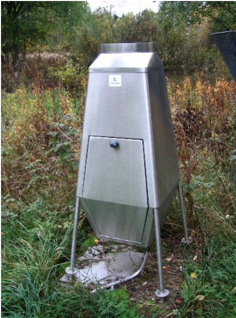
Figure 13. The “Ritva” collector for deposition. This collector is warmed in winter.
