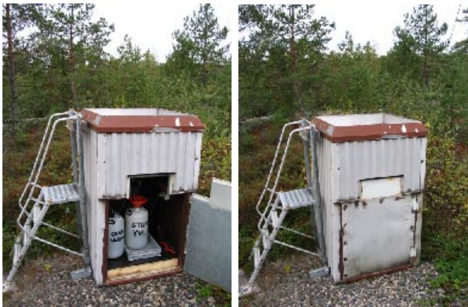
Figure 12. The large-area collector for deposition at Olkiluoto.
