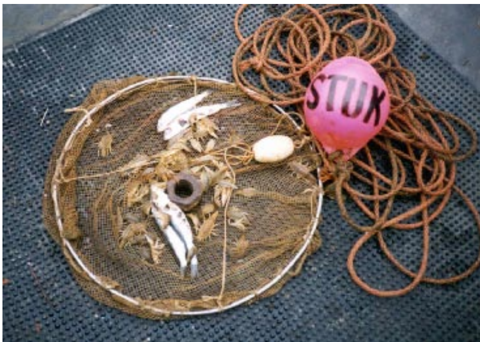
Figure 31. A bait net for the sampling of Saduria entomon .
