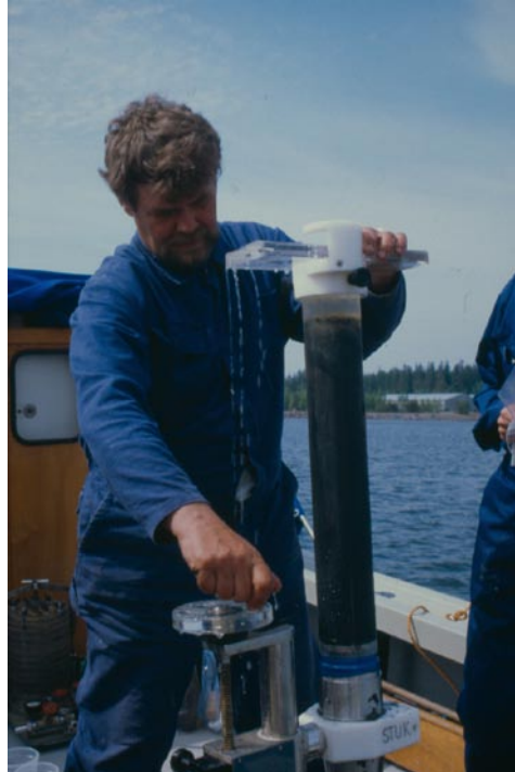
Figure 25. Sectioning apparatus of Gemini Twin Corer.
