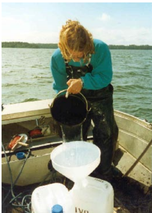
Figure 20. Water sampling with pail and funnel.
