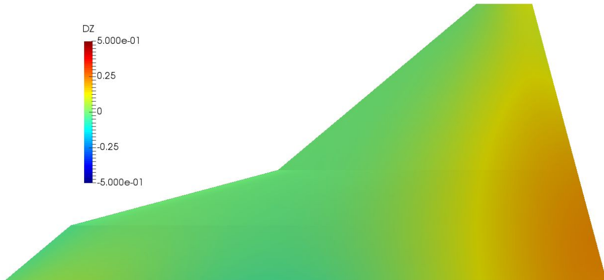
Fig 4.92 Mean camber surface of the transonic-constrained cranked wing
