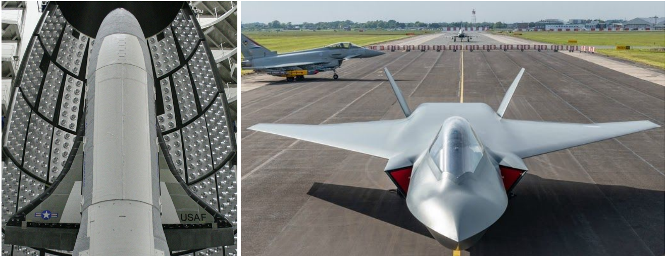
Fig 2.1 X-37B gliding re-entry vehicle, Boeing[40] and UK Tempest fighter concept, BAe Systems[41].
