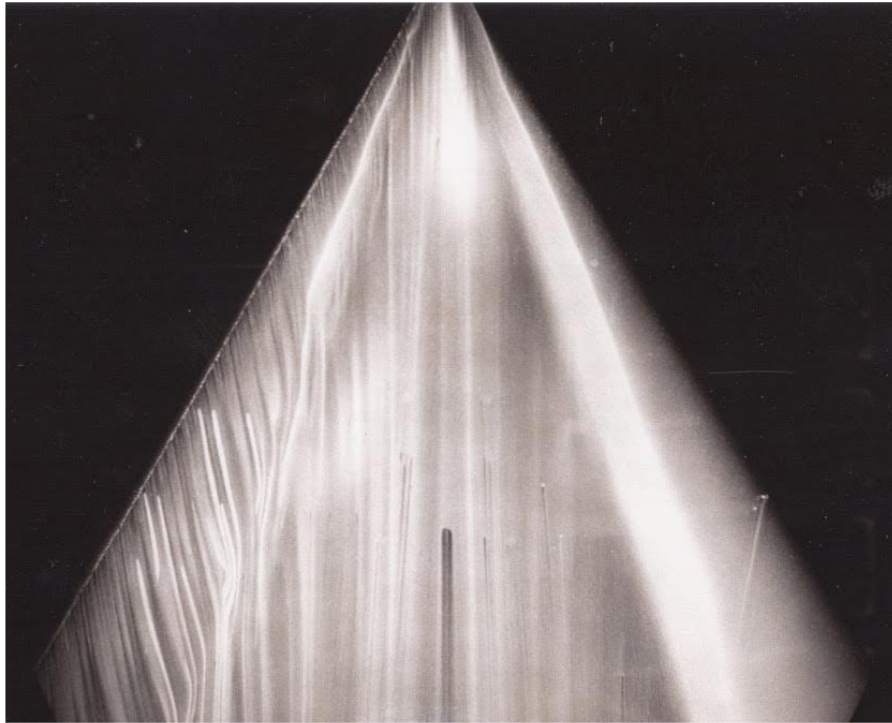
Figure 2.3 Oil flow Photograph by Mason of cambered wing at M=1.62 , \alpha=12 during testing for[33]. Kindly scanned from the original Polaroid, courtesy of Mason[47].
