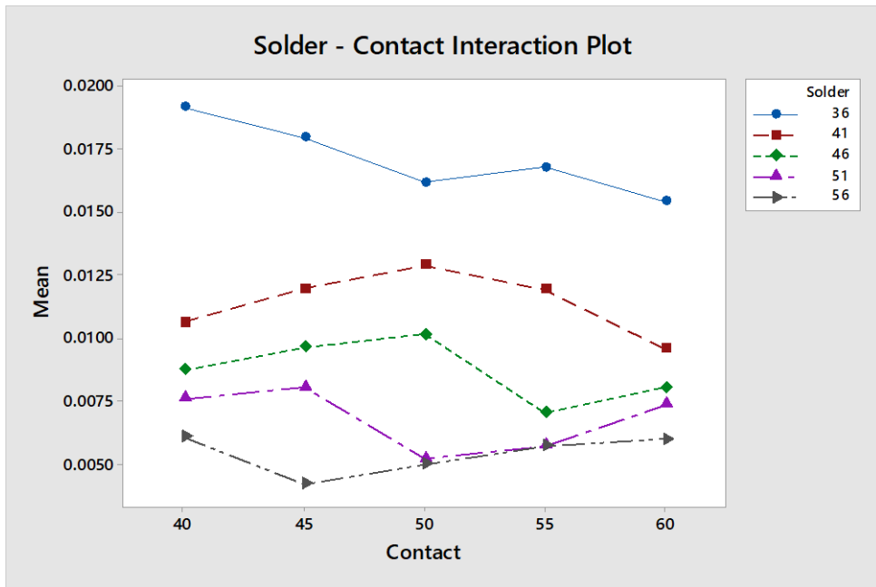
Figure 7.24: Solder-Contact interaction plot for Silver-Aluminium Combination
