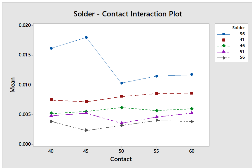
Figure 7.35: Solder-Contact interaction plot for Aluminium-Silver Combination
