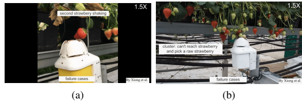
Fig. 2. State-of-the-art strawberry picking head [7]: although this sophisticated design can successfully pick most of the isolated strawberries, it fails to pick (i) some of them due to a large error in the planned target position 2a, or (ii) all the occluded strawberries 2b.
