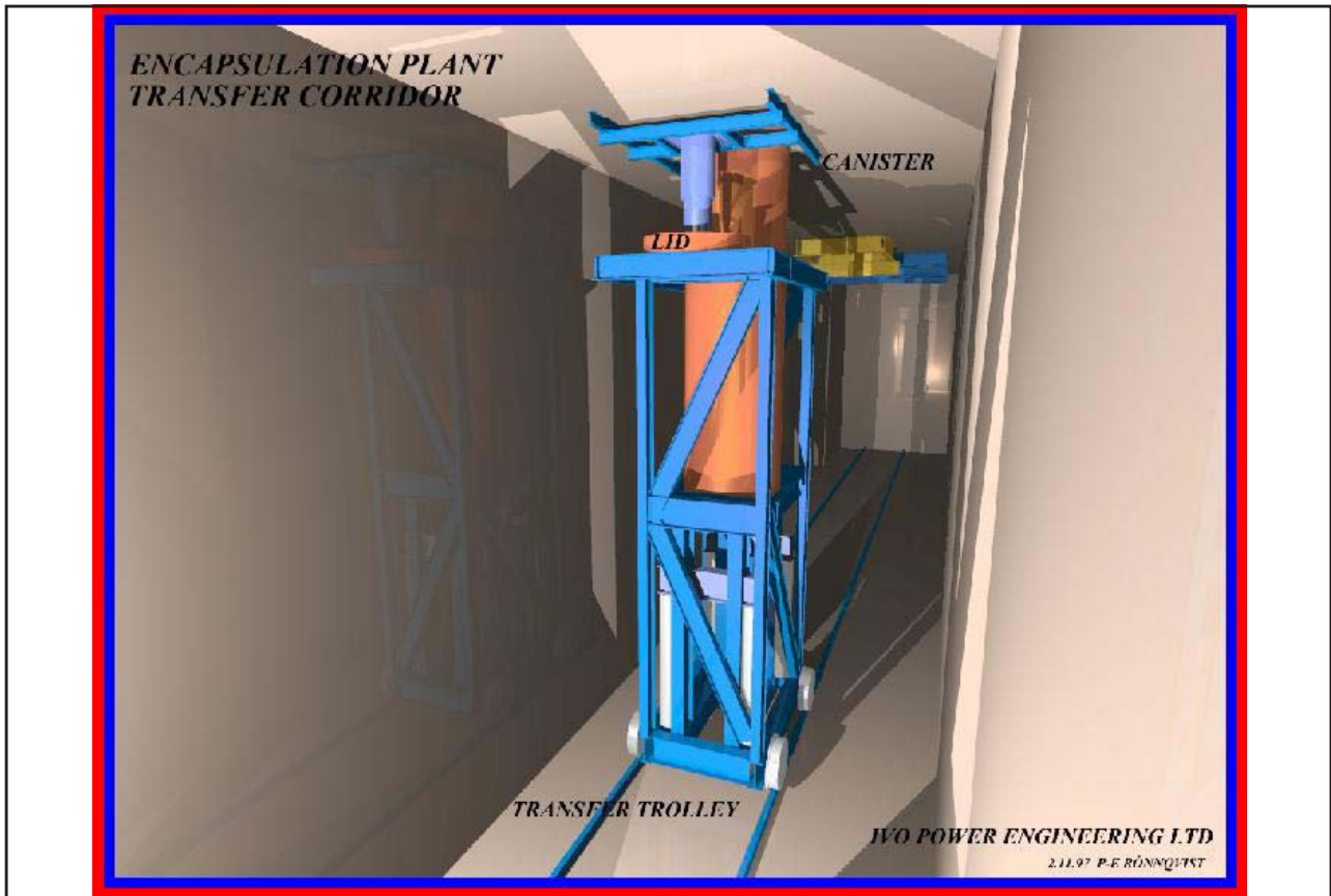
Figure 8. Transfer trolley and transfer corridor of the canister.
