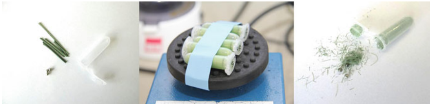
Fig. 4.1 Sample grinding is accomplished by combining desiccated leaf material and metal beads into a 2-ml tube ( left panel ) and taping sample tubes to a standard vortex mixer ( middle panel ). Grinding is complete when a fine powder is produced. The presence of unground tissue with the powder does not affect the quality of extracted DNA ( right panel , and example data in Chap. 8)
