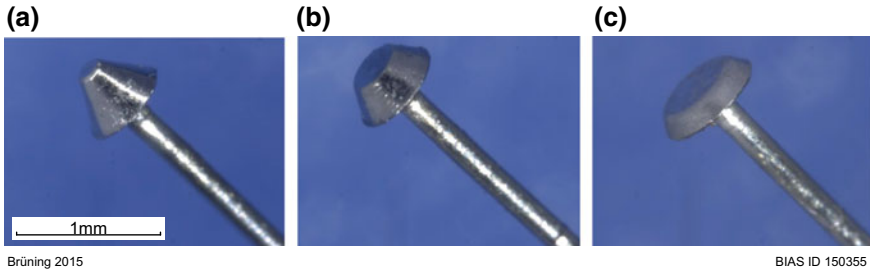
Fig. 2.9 Part after closed die forming using different averages of natural strain [Brü16b]
