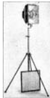
Fig. 2.5 – A double-carbon arc unit manufactured in Germany.
