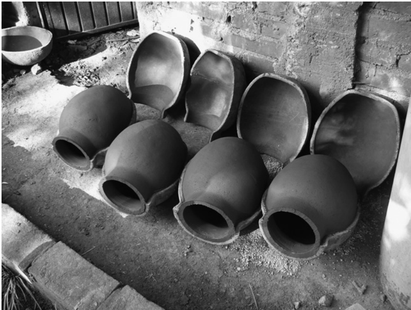
Figure 27. Ollas made with two vertical halve-molds in San Juanico.
