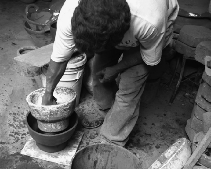
Figure 26. Process of vessel forming by molding.
