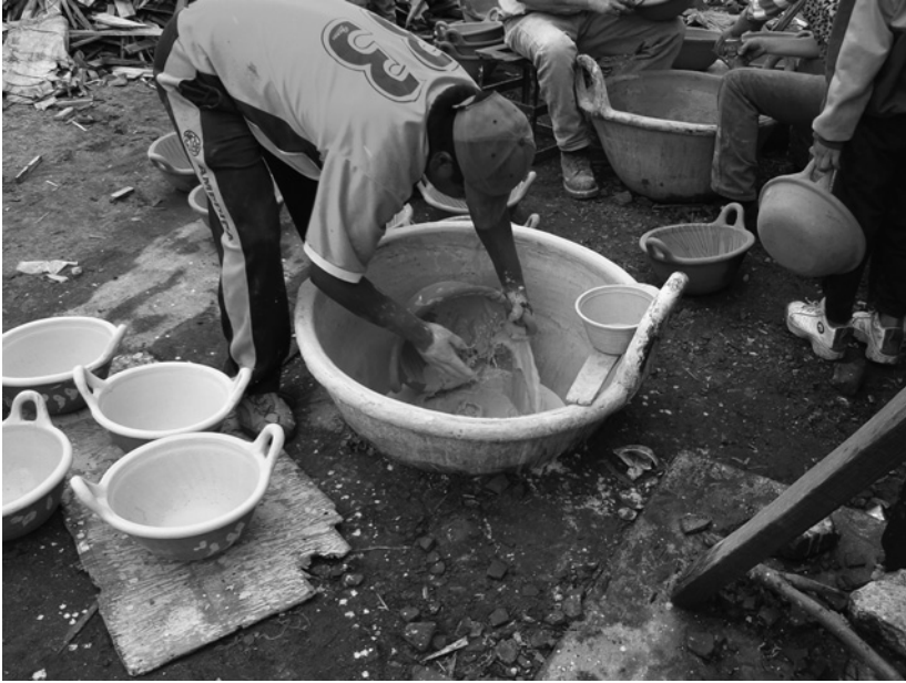
Figure 33. Application of greta on vessel before the second firing in Amozoc (Foto by Hermann Stützle).
