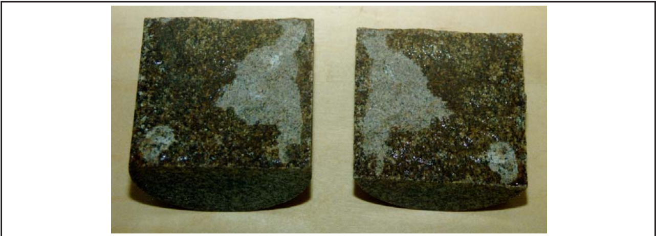
Figure 4. Flow wetted fracture surfaces at time t=t_1 after an instantaneous water injection input from the upper boundary (dark area is wet).
